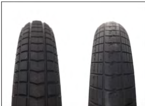
Fig. 8: Optimum tyre tread (left); Worn tyre tread (right)
