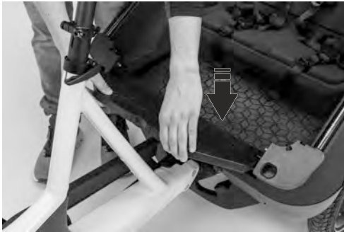
Fig. 22: Fold out the footboard
