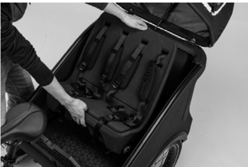
Fig. 39: Lift out child seat
