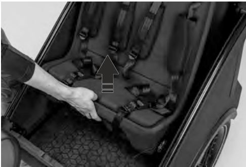
Fig. 38: Lift child seat at the front
