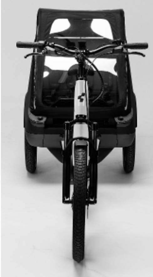
Fig. 9: Stem and handlebars correctly aligned
