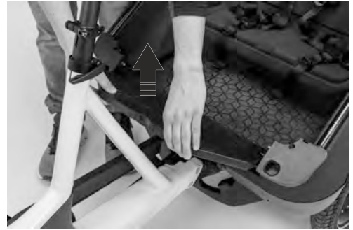
Fig. 24: Fold in footboard
